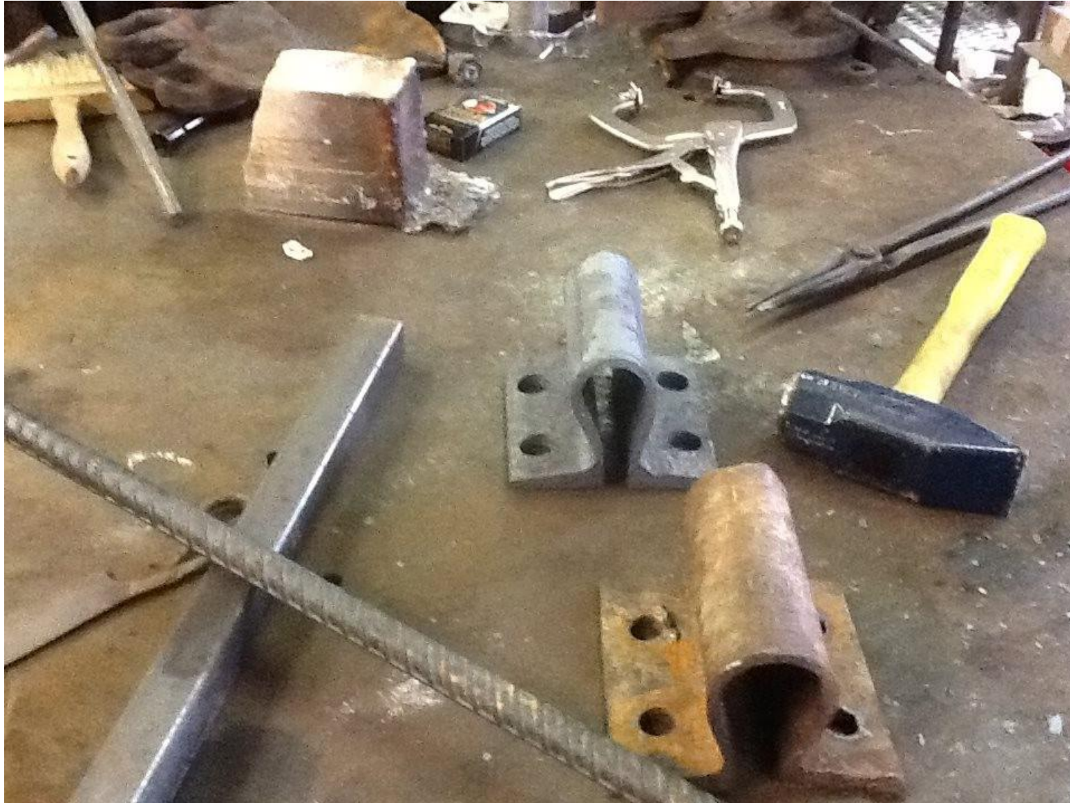
Replica attachments for the overhead lateral bracing had to be made. Original attachment in lower portion of photo, replica is above.
