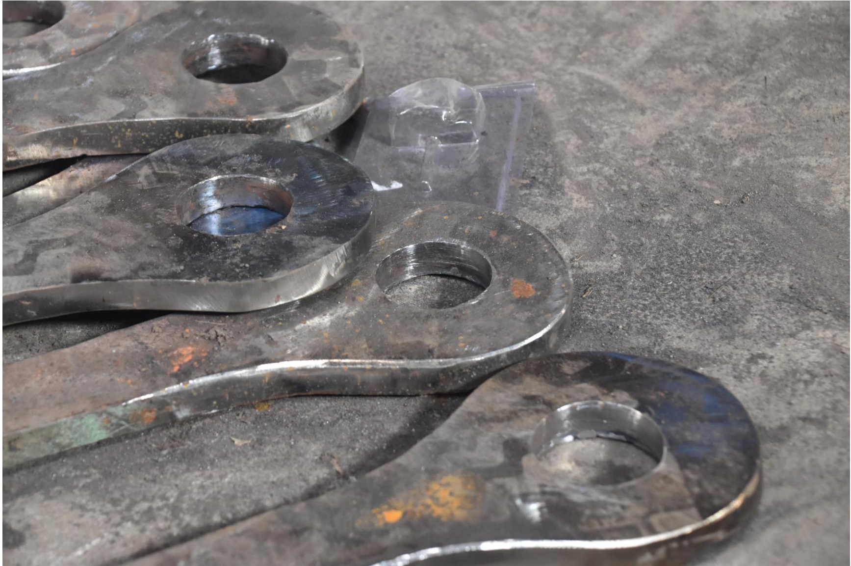
Shop Repairs (Pad Welding For Section Loss)
