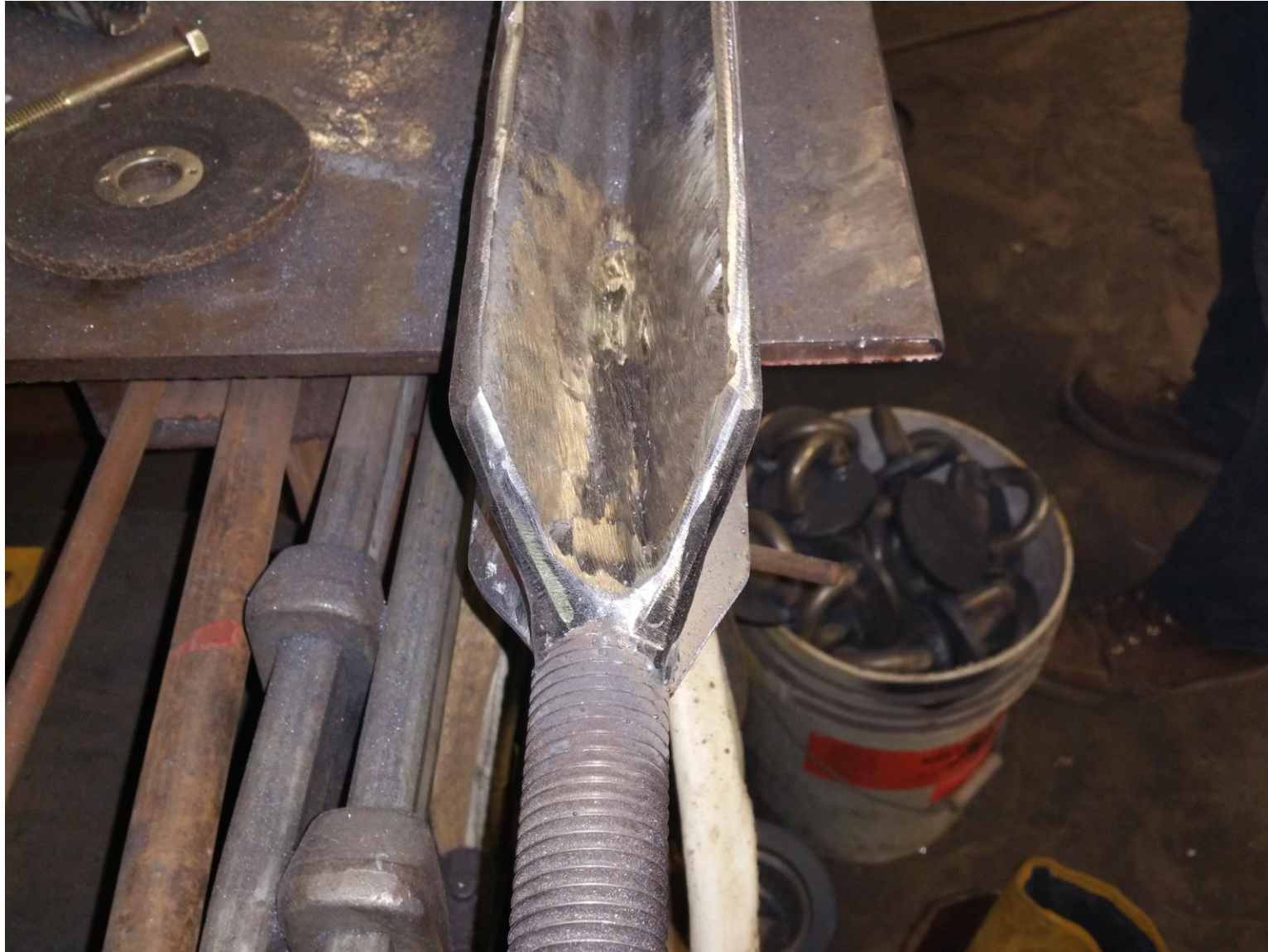
Replica Star iron (cruciform) fabrication.
