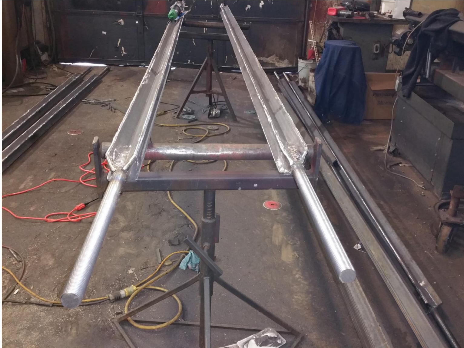
Replica Star iron (cruciform) fabrication.
