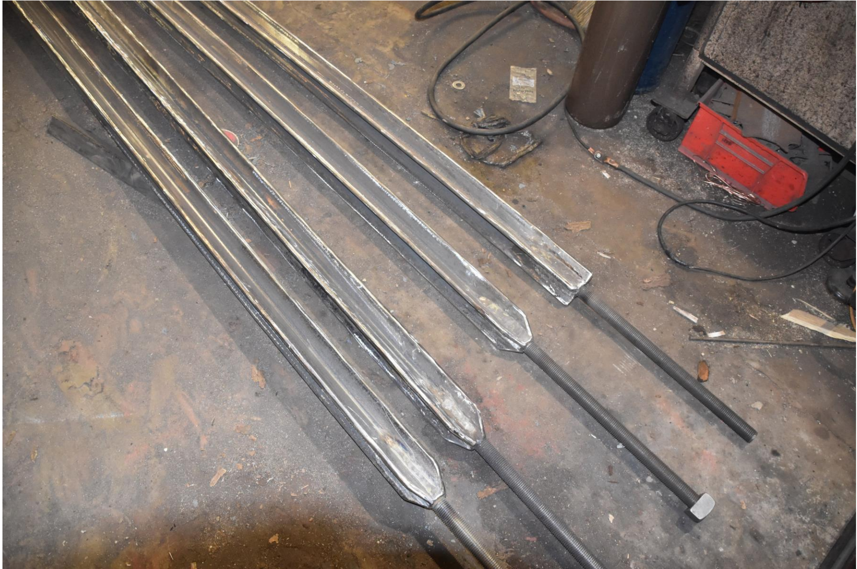
Replica Star iron (cruciform) fabrication.
