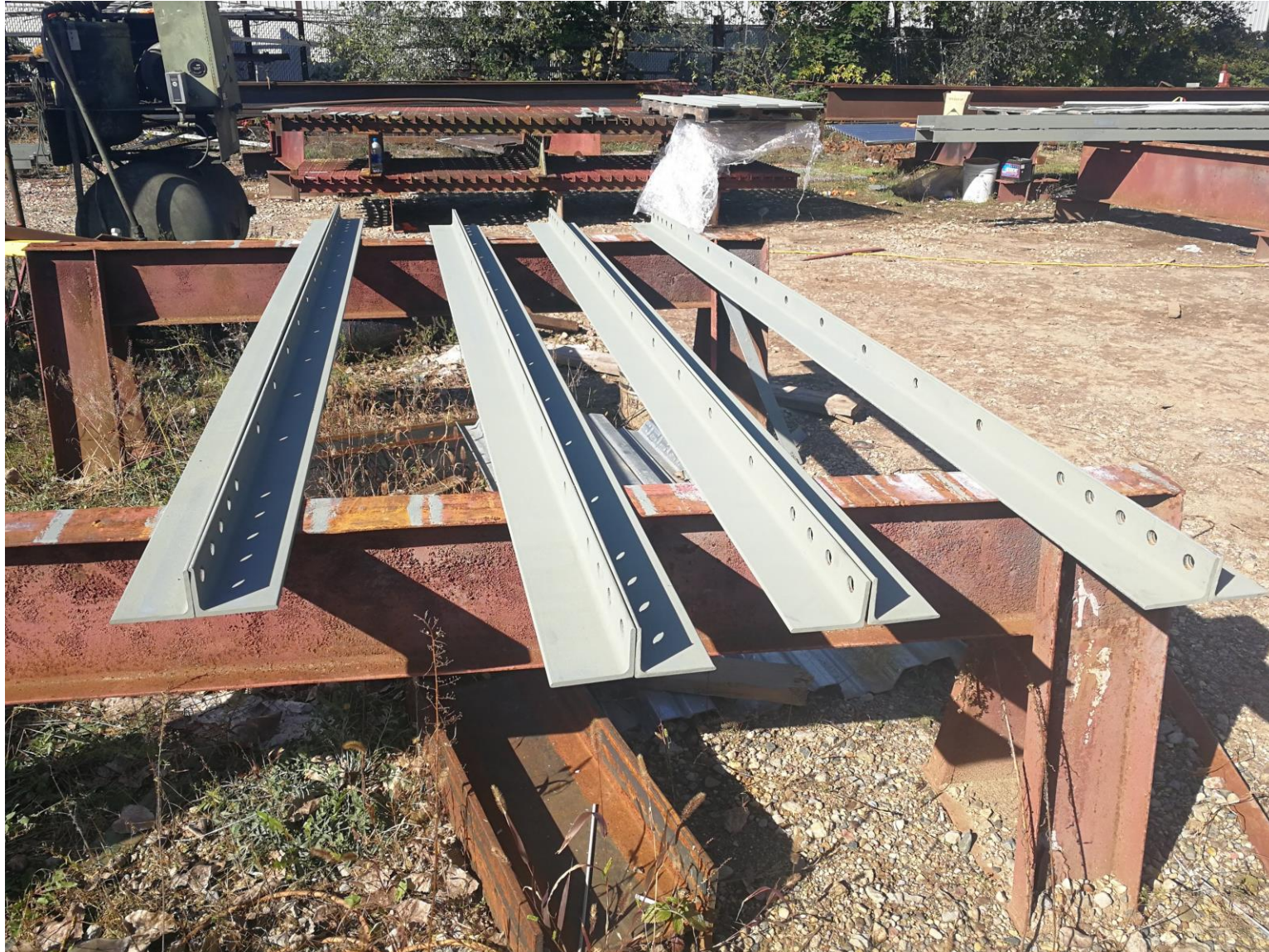
Angle for replacement bracing.
