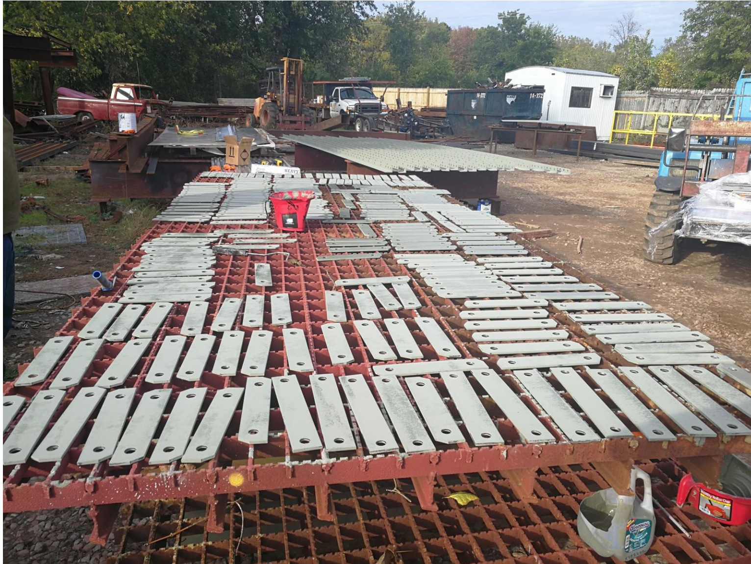
Lacing bars for replacement bracing.
