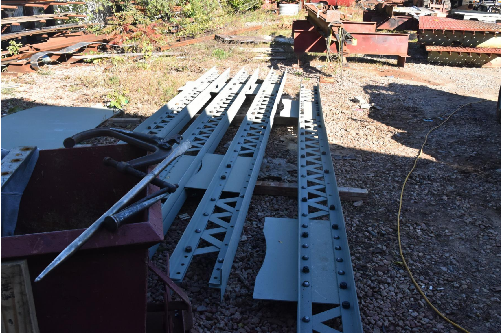
Completed replica bracing beams.
