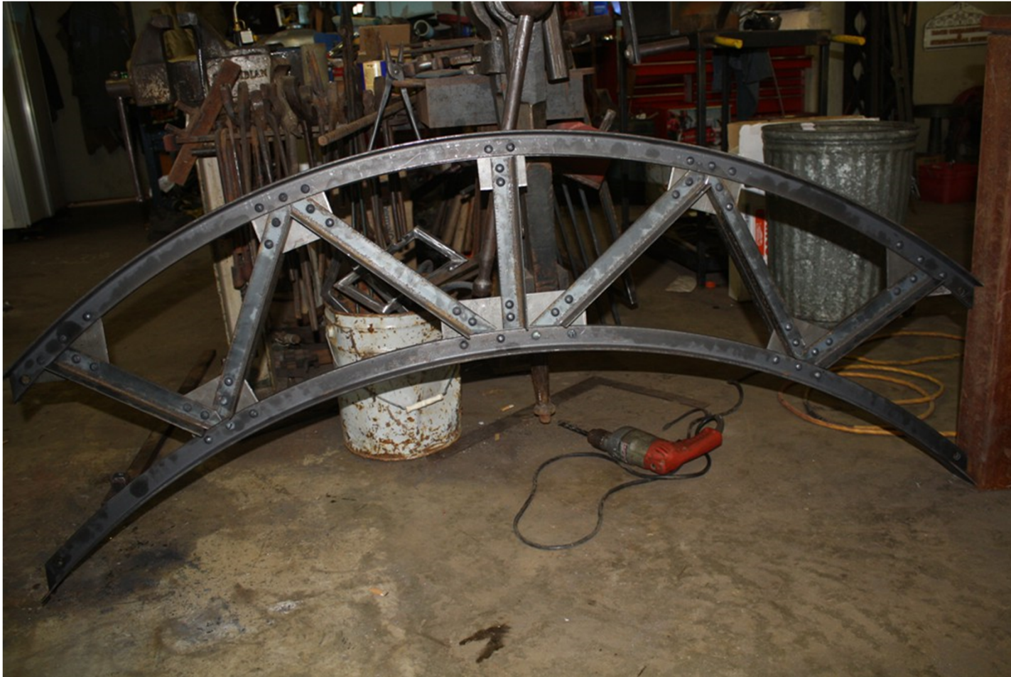
Riveted arches prepared in the shop.
