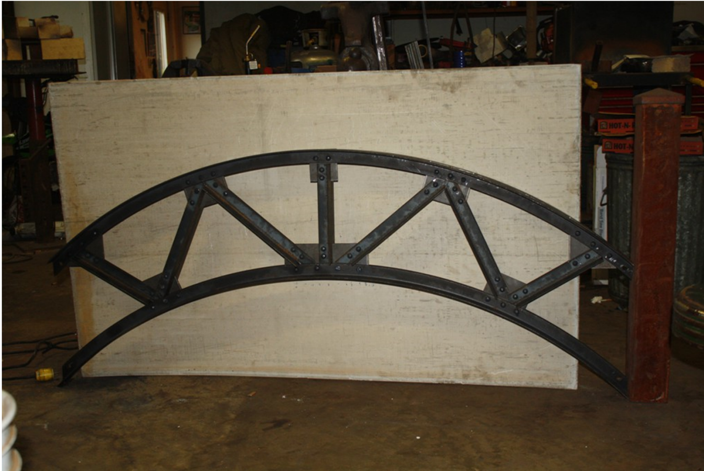
Riveted arches prepared in the shop.
