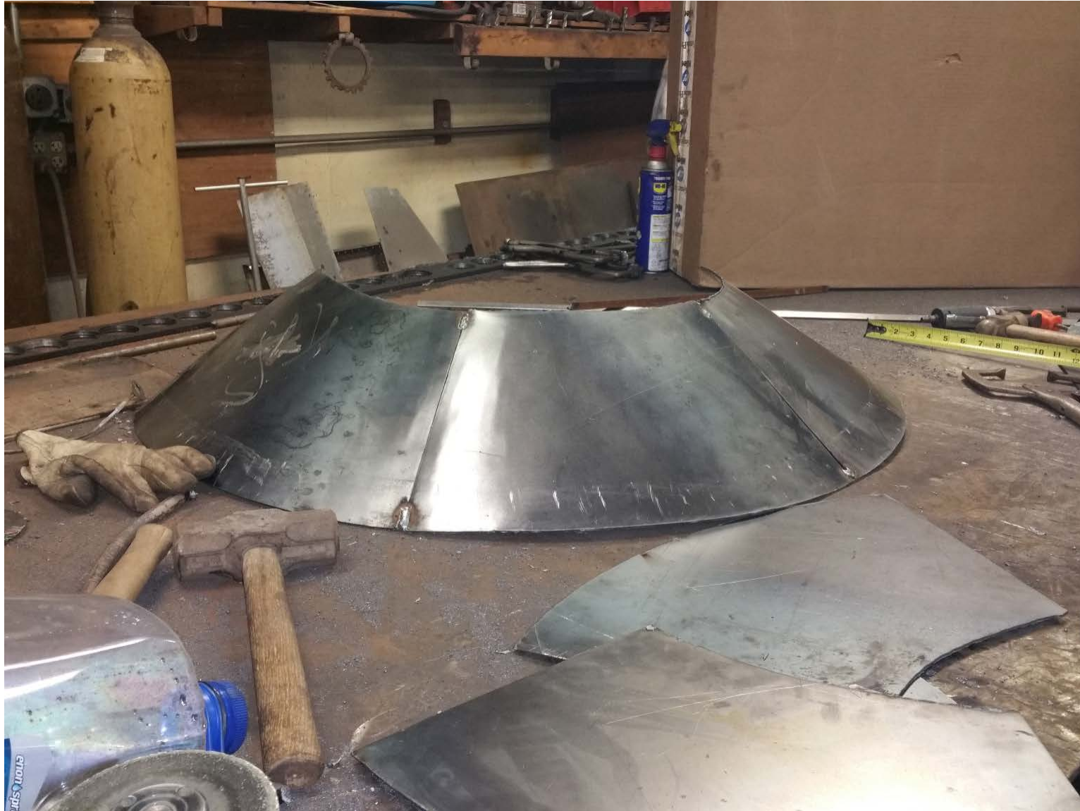
Fabrication of replica chimney cap.
