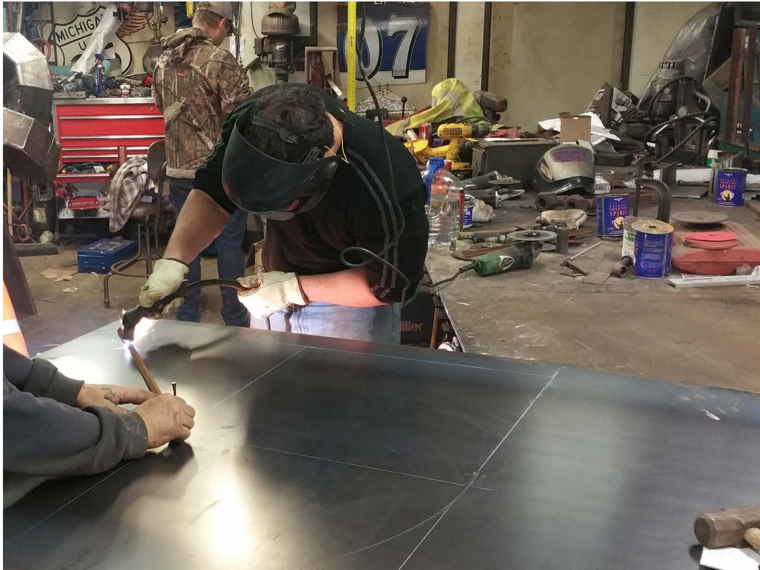
Fabrication of replica chimney cap.
