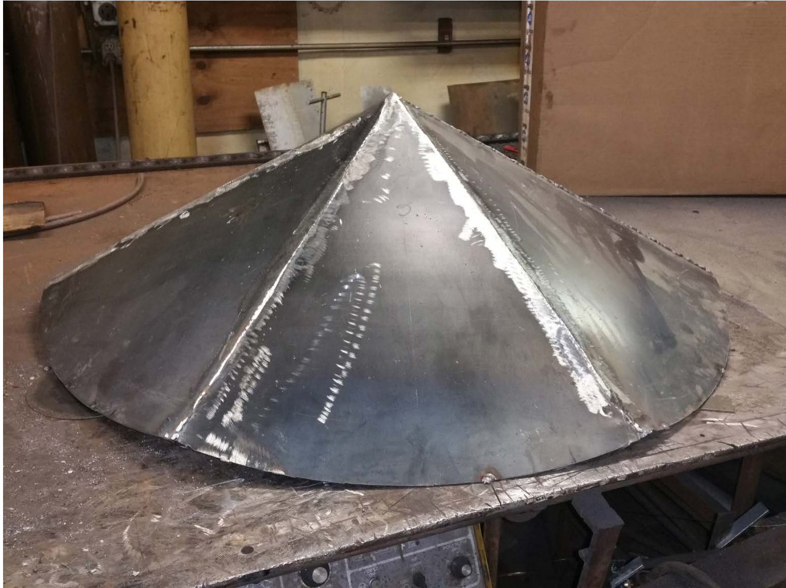
Fabrication of replica chimney cap.
