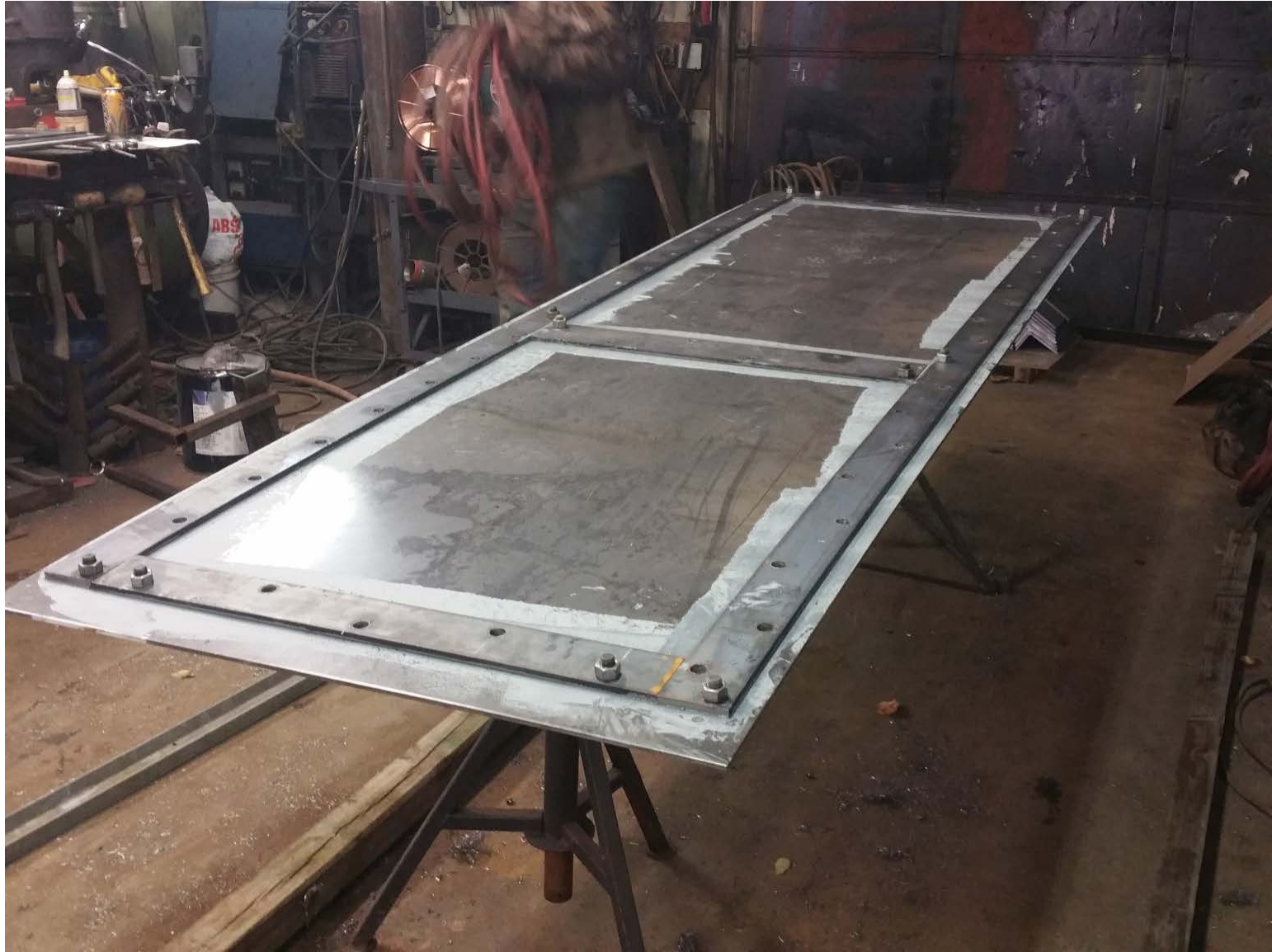
Shop fabrication and riveting of replica doors.
