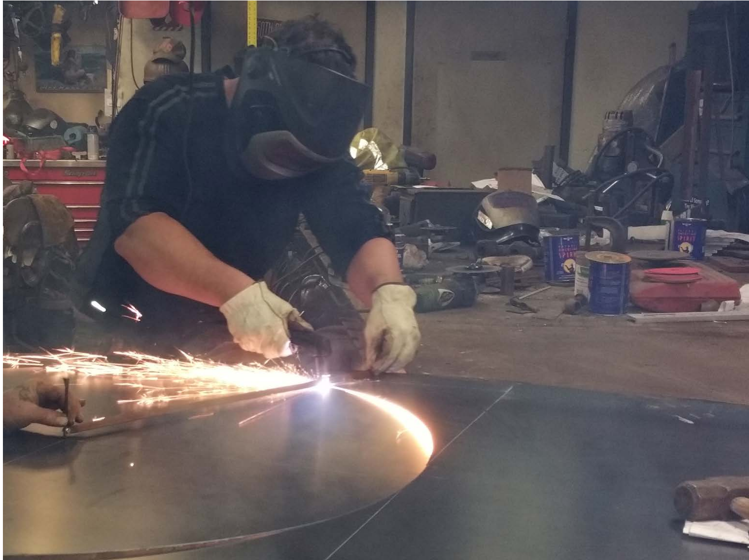
Fabrication of replica chimney cap.
