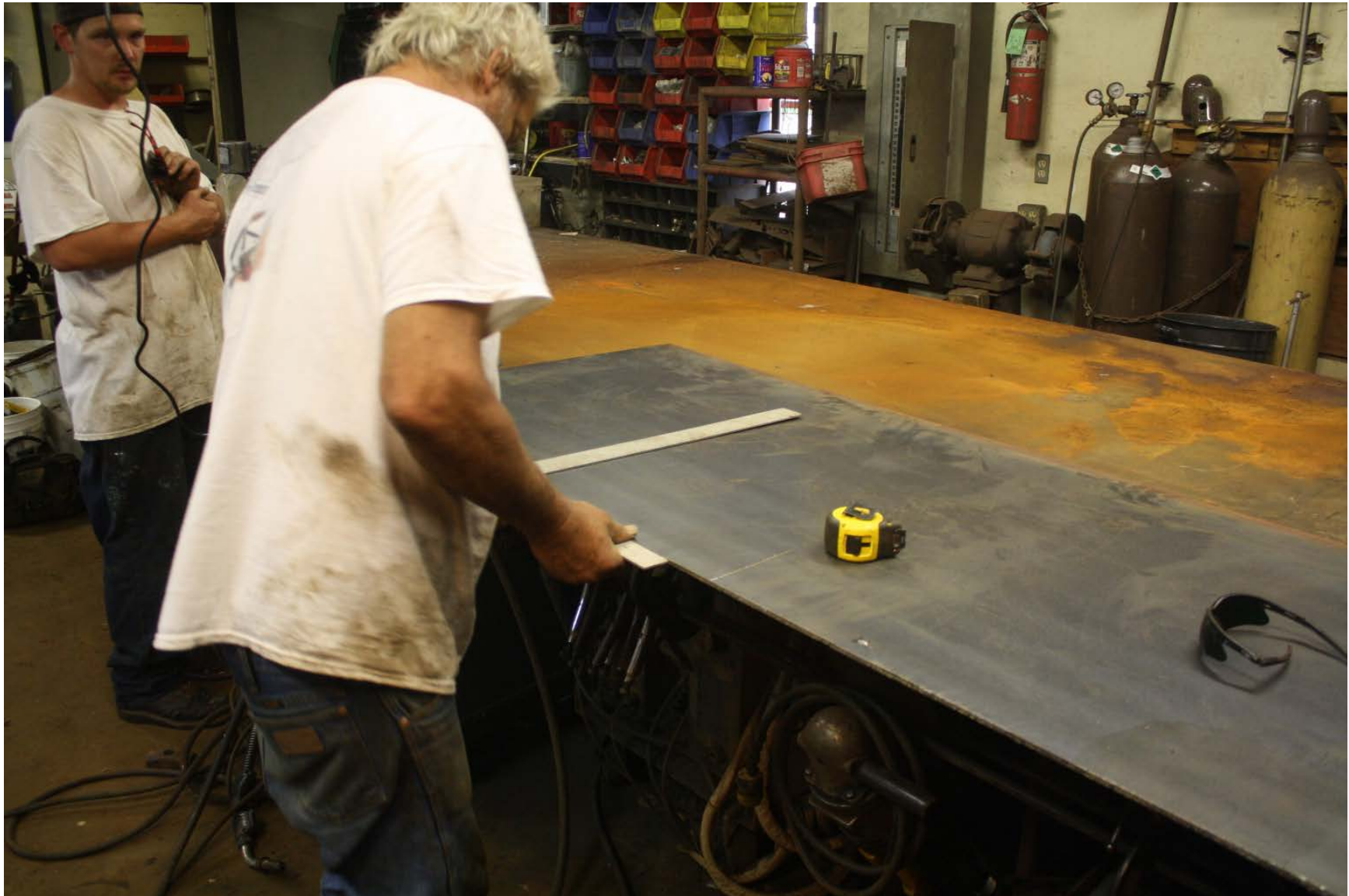
Shop fabrication and riveting of replica doors.
