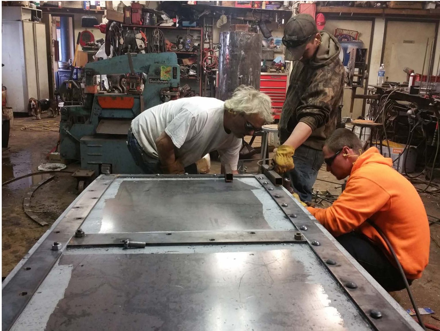
Shop fabrication and riveting of replica doors.
