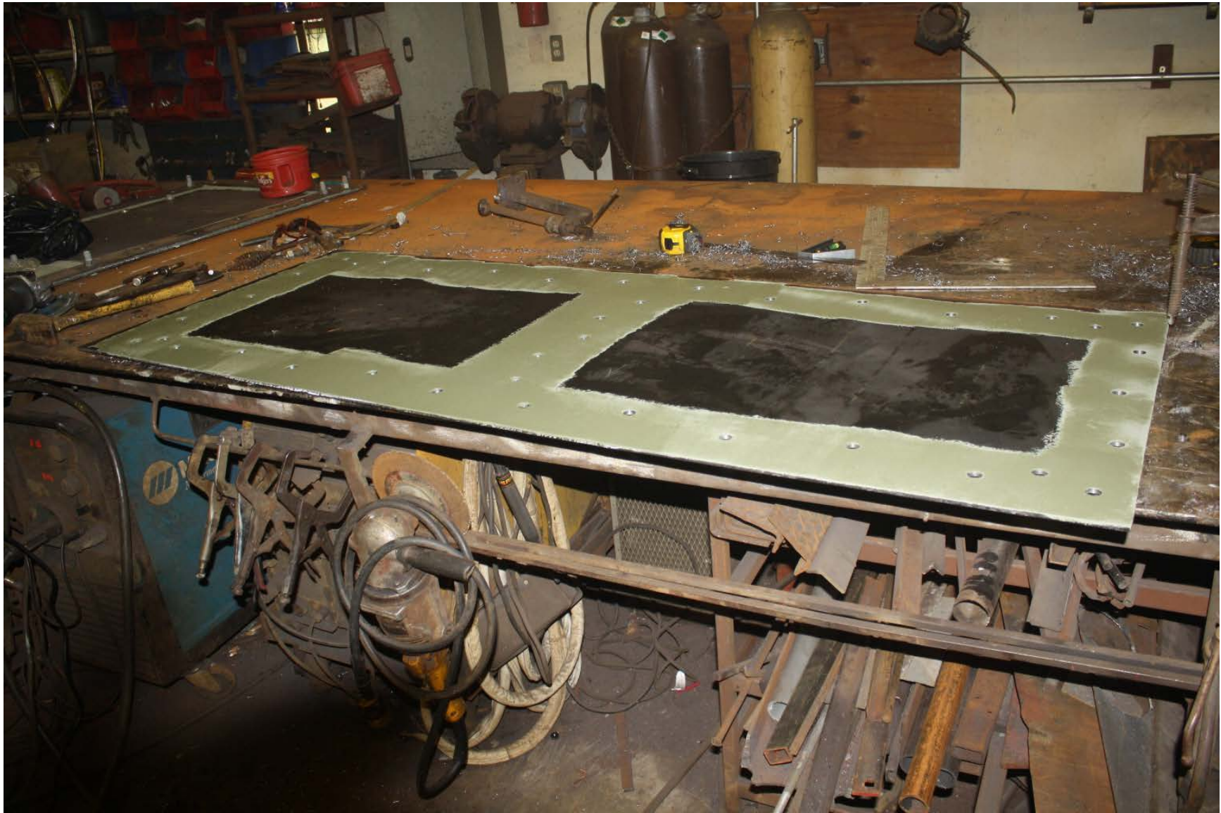
Shop fabrication and riveting of replica doors.
