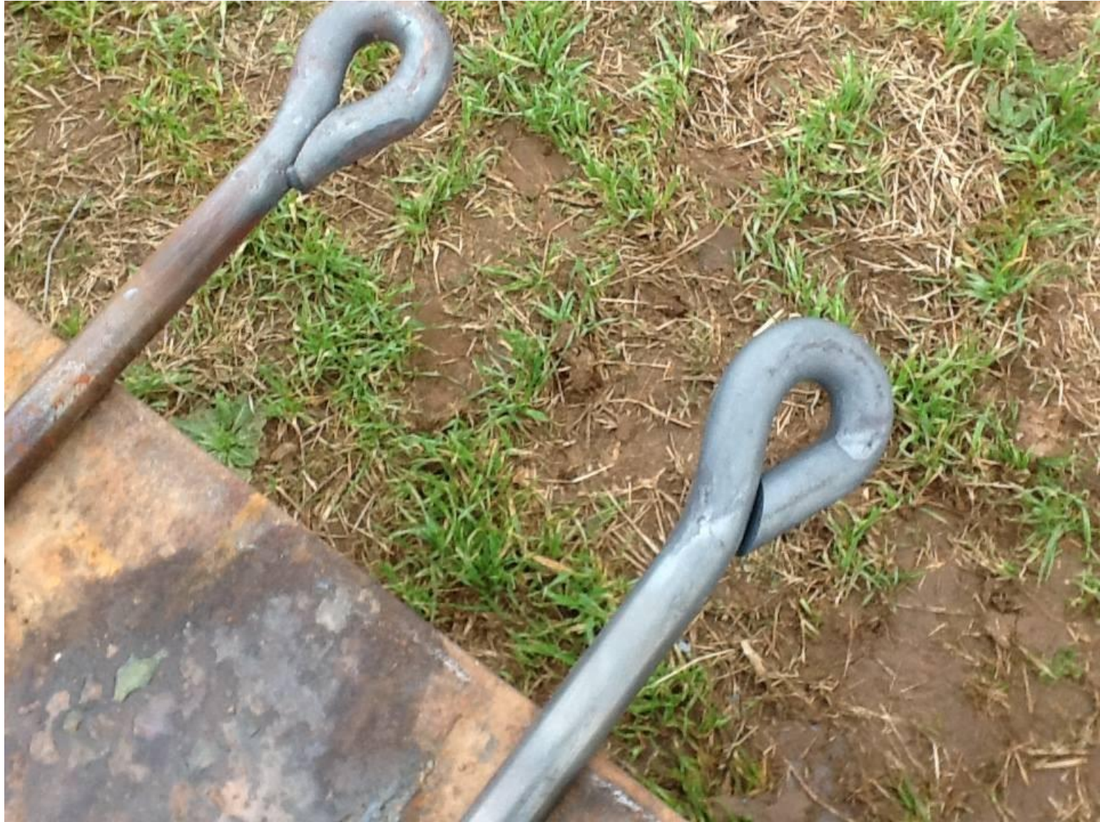
Fabricating a replica loop-forged eyebar.
