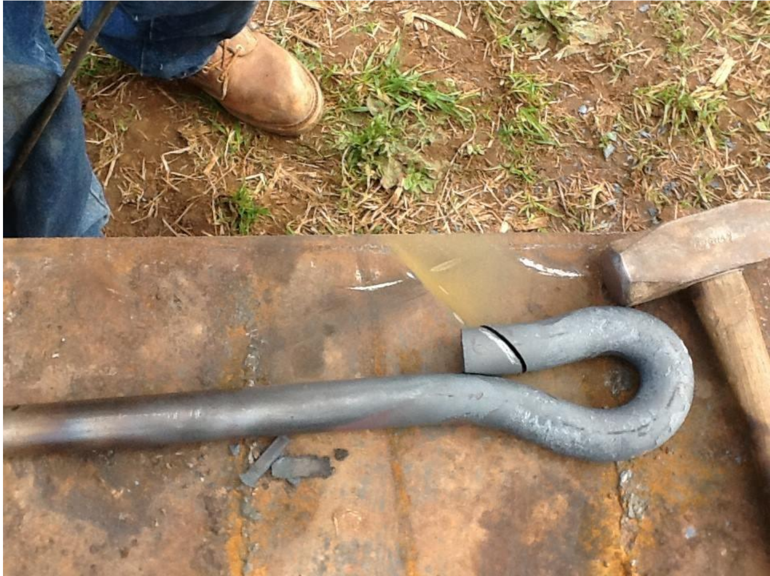
Fabricating a replica loop-forged eyebar.
