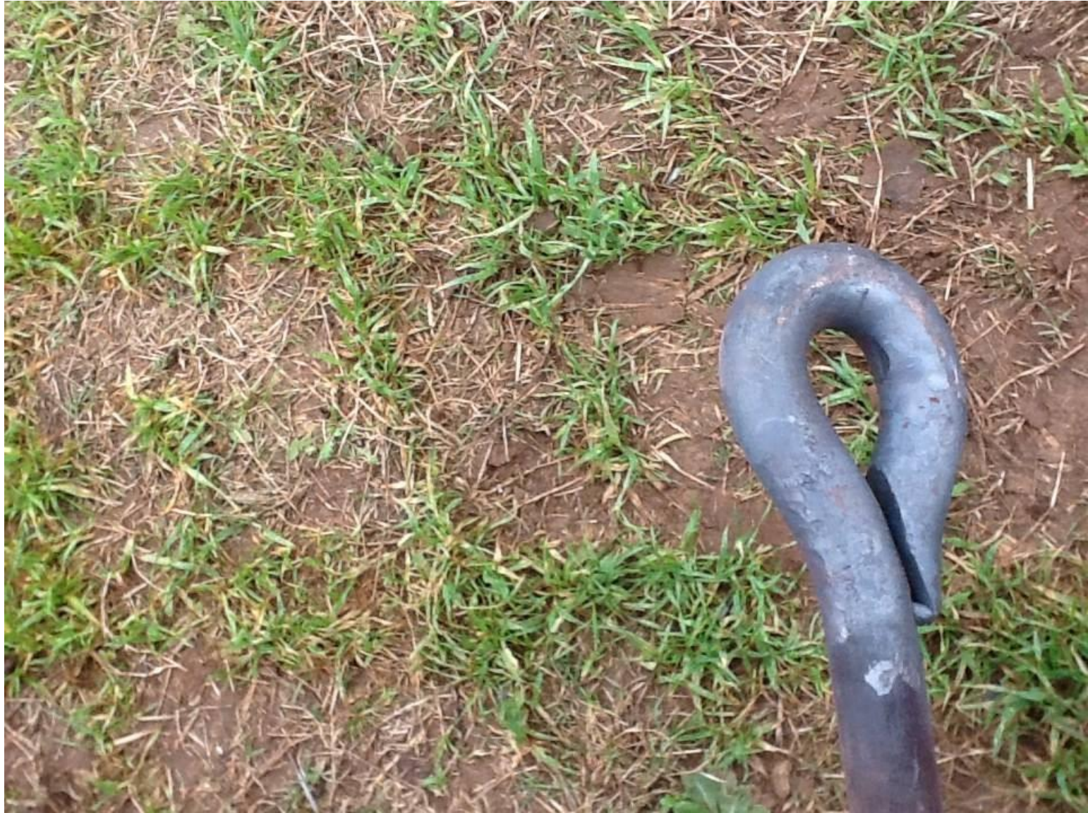
Fabricating a replica loop-forged eyebar.
